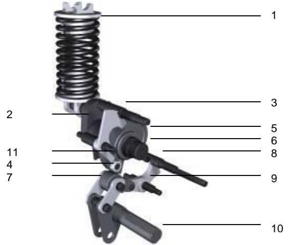
Fig. 6-9: Breaker Closed and Closing Spring Charged
