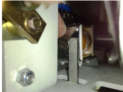
Fig. 5-11A: Cradle Electromagnetic Interlock
